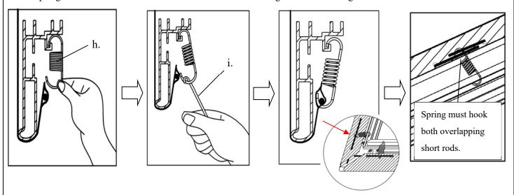
Begin by first attaching the center points on both vertical (left/right) sides, *steps 1-2*. Then the center points on both horizontal (top/bottom) sides, *steps 3-4*. Once all center points have been secured, make sure the screen material is still within the marked areas before proceeding to attach the next springs.
