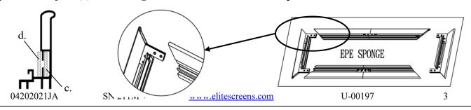
Step 5: Secure the elbow joints by fastening them with M4x7 screws (g), 4 at each corner.
