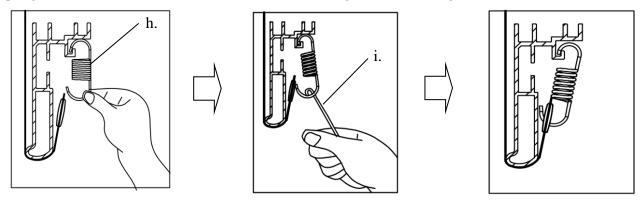
Begin by first attaching the center points on both vertical (left/right) sides, *steps 1-2*. Then the center points on both horizontal (top/bottom) sides, *steps 3-4*. Once all center points have been secured, make sure the screen material is still within the marked areas before proceeding to attach the next springs.
