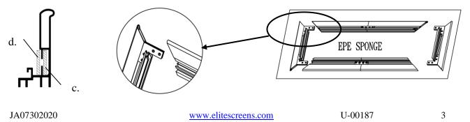
Step 5: Secure the elbow joints by fastening them with M4x7 screws (g), 4 at each corner.
