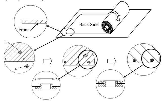
**Step 7:** Carefully and gently place the assembled frame on top of the screen material in the marked areas as shown below. Make sure to not allow the angle edge of the frame to come in direct contact with the screen material to avoid puncturing it.
