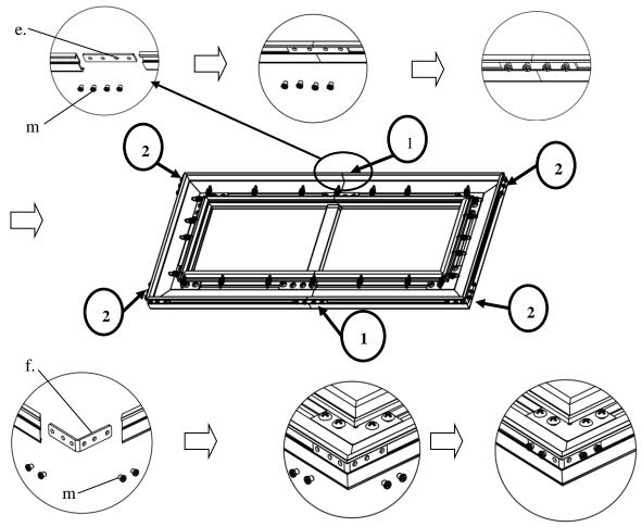
**Step 11**: Install the *angle cover* (*n*) on each corner of the frame using the *M4x4 screws* (*m*). Note: The angle cover screws holes align with the screw holes on the elbow joint.
