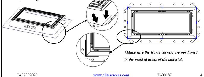
**Step 8:** Hook one end of the spring and secure inside the groove of the frame, use the *spring hook* (*h*) to attach the spring to the hole located on the screen material's outer edge in the following order.
