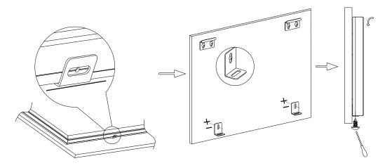
**Step 14.** Once the fixed frame screen is secure on the wall, place a screw at the bottom connecting the screen to the bottom bracket.
