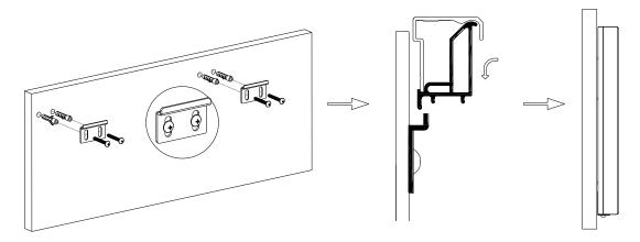
**Step 13.** Repeat the same process for the Bottom Brackets (K) by marking the drill-hole area on the wall where they will be installed. Make sure the brackets are flipped the opposite way mirroring the top brackets. Line up the bottom wall brackets with the drilled holes on the installation location and screw them in using a Phillips screwdriver as shown below.
