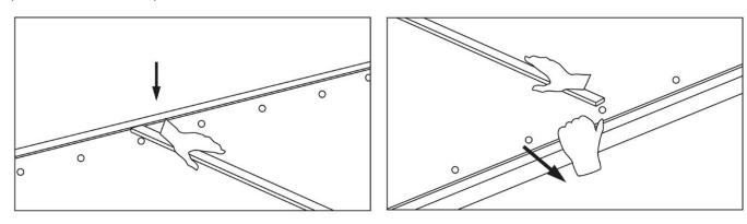
**Step 10.** Once the corners and center support bar are secure, continue attaching the reminder of the Springs (B) to the material. Connect the center of the vertical and horizontal portions of the material, then work your way around the rest of the frame.
