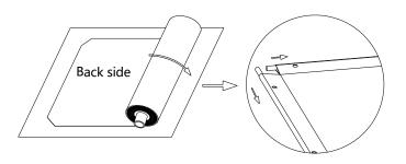
flat. Careful not to snag on the holes at the edge of the material during this process; forcing the rods may damage the screen material.
