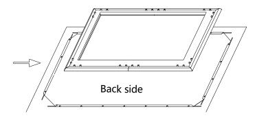
Step 7. Carefully place the assembled frame on top of the material and slowly fold the edges over the frame as shown. Make sure to not allow the angle edge of the frame to come in direct contact with the screen material to avoid puncturing it.
