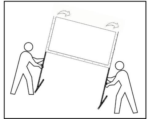
3. Unlatch the hinged support bars and fold down other half of the legs.
