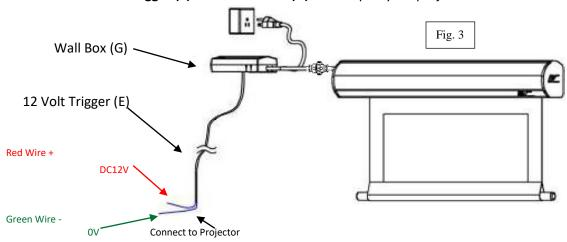
6. <u>Wireless 5-12 volt trigger</u> (Item F, Fig 4): The RF remote control serves as a dual purpose, independently as a handheld remote control, or in conjunction with the Wireless 5-12 volt trigger cable. The radio frequency technology can be programmed to send a wireless signal to synchronize its drop/rise with the projector's power cycle.
