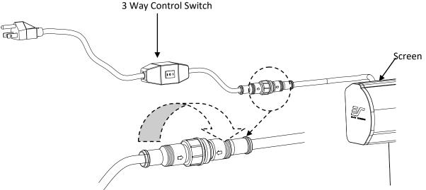
2. Connect the Wall Box (G) to the screen as shown below.
