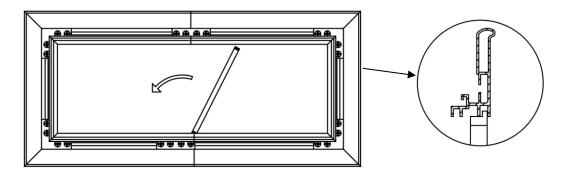
**Step 10:** Hook one end of the spring and secure inside the groove of the frame, use the *spring hook* (h) to attach the spring to the hole located on the screen material's outer edge in the following order.
