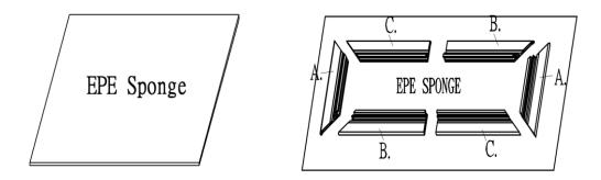
Step 3: Insert center joint (a/b) connectors into one-half of the horizontal frame (B/C) and secure with the M4x7 screws (M) as shown in the illustration below.
