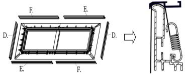
Connect edge trim frames (e/f) together using the M4 center joint (e) and secure with four of the M4x4 screws (m) as show in Step 1. Repeat for other side.
