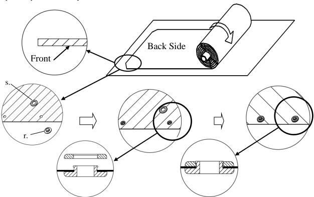
**Step 7:** Carefully and gently place the assembled frame on top of the screen material in the marked areas as shown below. Make sure to not allow the angle edge of the frame to come in direct contact with the screen material to
