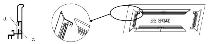
Step 5: Secure the elbow joints by fastening them with M4x7 screws (g), 4 at each corner.
