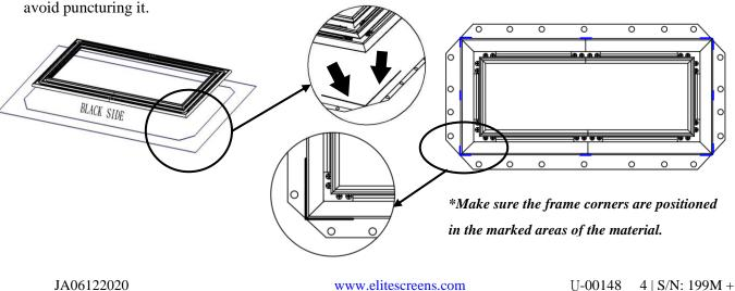
**Step 8:** Hook one end of the spring and secure inside the groove of the frame, use the *spring hook* (h) to attach the spring to the hole located on the screen material's outer edge in the following order.
