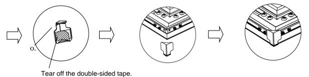
**Step 12**: Install the **springs** (q) in each middle area to further support the bezel trim edge frame.
