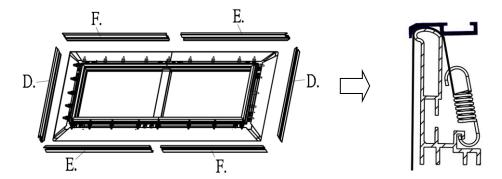
Connect edge trim frames (e/f) together using the M4 center joint (e) and secure with four of the M4x4 screws (m) as show in Step 1. Repeat for other side.
