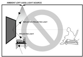
Note: Improper installation will result in light loss and produce a dark image. This is due to the projector's light reflecting in the wrong direction.
