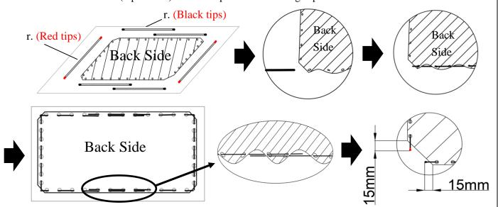
**Step 8:** Carefully and gently place the assembled frame on top of the screen material in the marked areas as shown below. Make sure to not allow the angle edge of the frame to come in direct contact with the screen material to avoid puncturing it.
