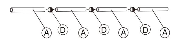
Disassemble the Top/Bottom posts by disjointing the straight joints.
