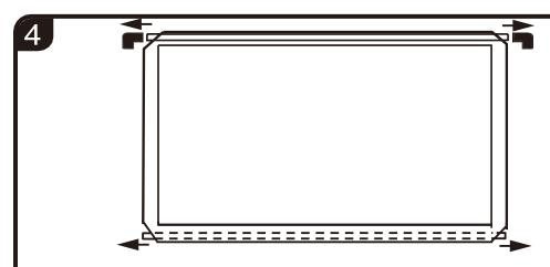
Remove the elbow joints at both ends of the top crossbar and slide both top/bottom crossbars out of the screen.
