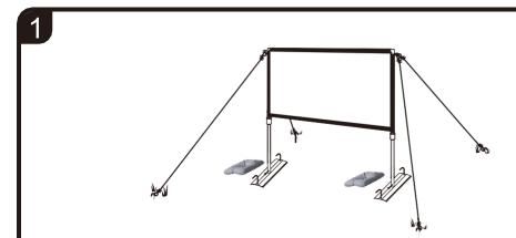
Remove the stakes from the tethering ropes and base. Then remove the tethering ropes from the screen.
