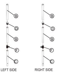
Disassemble the L/R posts by disjointing the straight and T-joints.
