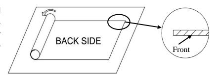
**Step7**: Carefully place the screen on top of the assembled frame as shown below. Make sure that the angular **edges** of the frame are not allowed to come into direct contact with the screen material to avoid puncturing.
