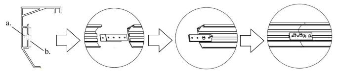
**Step 4:** Connect the *elbow joints* (*c/d*) to the top and bottom sections of the vertical frame. Once inserted, connect the vertical sections to the horizontal frame sections. Make sure all holes are in alignment and the frame pieces are flush (no gaps). They should form perfect right angles.
