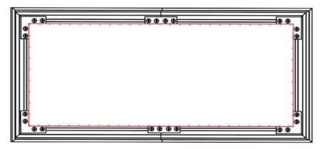
**Step 8:** Insert the rods(r) through the sleeves according to their corresponding lengths on each edge of the screen as shown below. The short rods (top/bottom) will overlap to secure a firm grasp in the middle areas.
