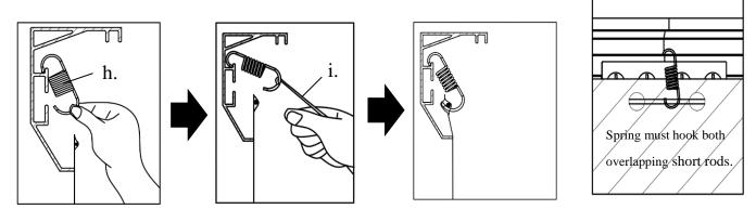
First connect on four corners, steps 1-4. make sure all four corners are fixed before proceeding with next spring.
