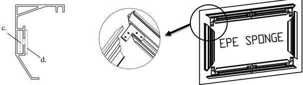
**Step 5.** Secure the elbow joints by fastening them with M4x7 screws (g), 4 at each corner.
