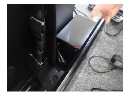
4. After removing the end cap, you will notice a metal box, directly behind the screen's material. This metal box houses the circuit board. Loosen and remove the screws that hold the cover of this metal box.
