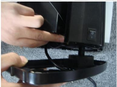
14. Be sure to turn the end cap at a 45 degree radius upwards when replacing it so that the motor peg can insert back into the cap to allow the cap to seal back in to its place.
