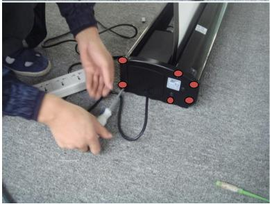
2. REMOVE the 6 screws as shown on the picture marked in red.
