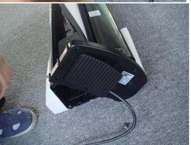
15. Fully extend the power cord out of the casing before completely sealing the end cap back in to place.
