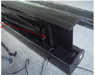
1. Raise the screen about 2', then unplug the power cord. VERY IMPORTANTLY: Use rope to tie the screen from both ends after raising it. When removing the end cap, the screen will spring open and can cause serious injury and can permanently damage the screen.
