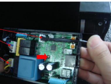
8. Detach indicated wires from the circuit and remove the small screws that hold it in place. Then, remove the circuit board. Do the reverse of step 8 instructions to replace the new circuit board.
