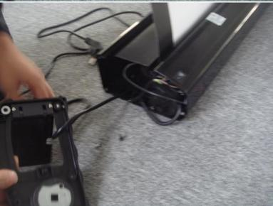
3. Remove the end cap. (careful not to pull the motor)
