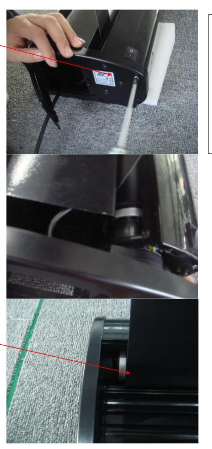
16. Put the end cap back in to place and tighten the end cap with the provided screws as shown in the picture.
