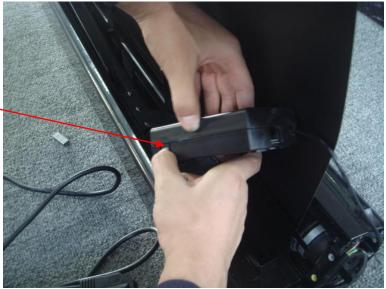
7. To open the circuit box, push in on the tab as shown in the picture and pull the box open with both hands simultaneously.
