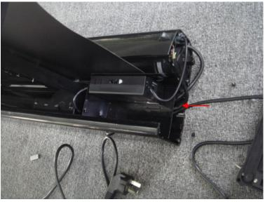
6. For easier access of the circuit board housing, push the power cord underneath the screen so that it is out of the way.
