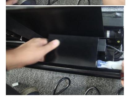
12. Put metal box cover back in to place and tighten with the screw and nut.
