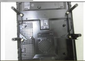
7. Water permeated into the specimen after IPX2 Test
