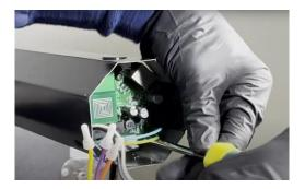
Remove the circuit board and replace with the new one. Next, move the switch to the "right" position for down/up screen type.
