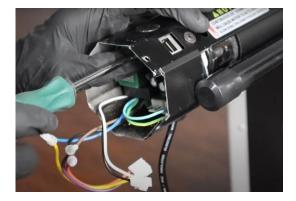
Plug both connection ports onto the new circuit board. Then, reattach and secure the endcap to the housing by fastening the screws on the side.
