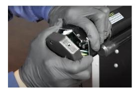
Unplug both connection ports from the circuit board. Then remove the three screws that fasten the circuit board to the housing.
