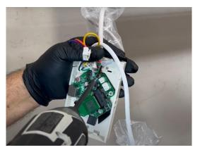
Before installing the new circuit board, move the switch to the "right" position for down/up screen type. Next, align the new circuit board with the back cover.
