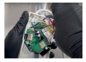
Plug both connection ports on the new circuit board. Then, Plug the screen into a power outlet and check that the circuit board lights up
