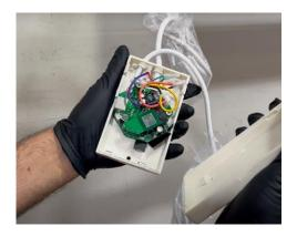
Unplug both connection ports from the circuit board. Then remove the three screws surrounding it.
