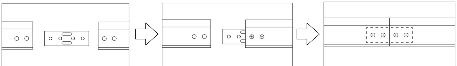
**Step 4.** Connect the *Elbow Joints (c)* to top and bottom sections of the vertical frame. Once inserted, connect the vertical sections to the horizontal frame sections. Make sure all the holes are in alignment and the frames pieces are flush (no gaps). They should form perfect right angles.
