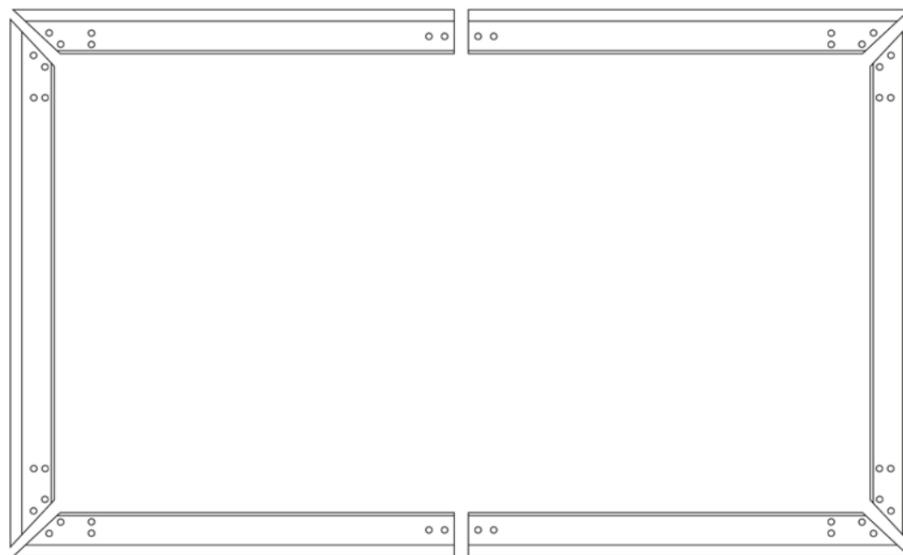
**Step 3.** Insert the *Center Joint (a)* connectors into one-half of the horizontal frame and secure with two *6x12mm Hex Screws (d)*. Once secure, connect the other half of the horizontal frame and fasten with two *6x12mm Hex Screws (d)*.
