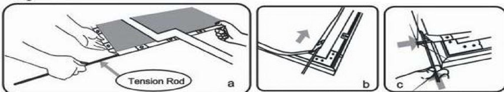
**Step 8.** Insert the *Springs (b)* into the grooves of the frame. Line them up with the corresponding holes in the materials edge. The shorter hook on each spring should be placed in the frame's groove, as shown below. For the correct amount of springs to place into the frame, please refer to the table listed below.
