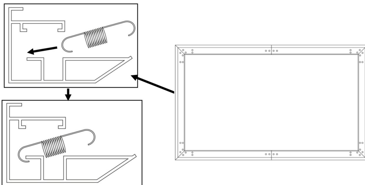
**Step 9.** With one end of the spring placed inside the groove of the frame, hook the *Spring (b)* through the hole located on the screen material's outer edge. **Be sure to hook the *Springs (b)* onto the *Tension Rod (k)* to avoid damage to the screen material.** Use the *Pull Hook (f)* when necessary. Attach the springs at the four corners (1).
