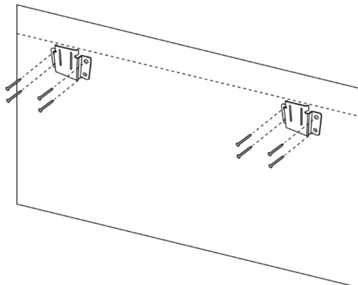
**Step 12.** Position the fixed frame screen onto the wall *Brackets (g)* as shown below and push down at the center of the top of the frame to secure.
