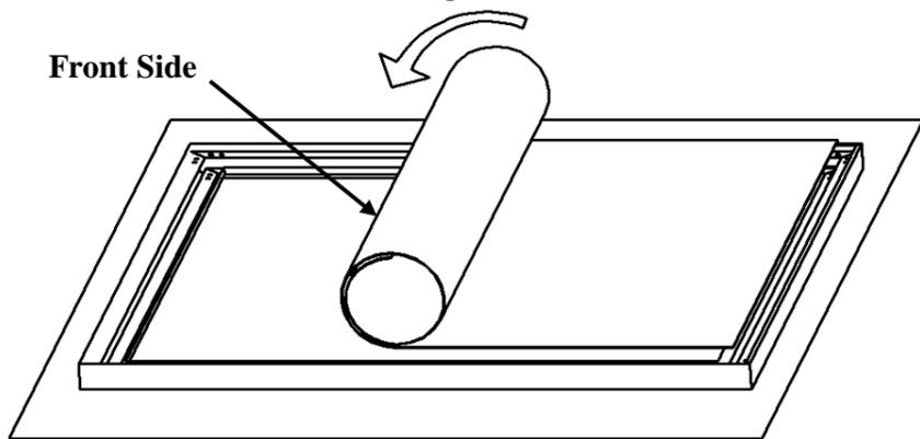
**Step 7.** Insert the four horizontal and two vertical *Tension Rods (k)* into the corresponding sides of the screen material, while keeping the material laying flat. Careful not to snag on the holes at the edge of the material during this process; forcing the rods may damage the screen material.
