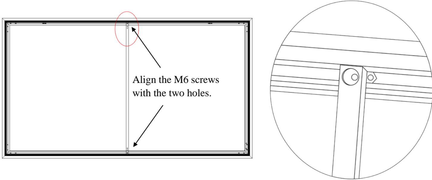
**Step 11.** After the *Center Support Bar (l)* is secure, connect the center of the vertical portions of the material (2). **Be sure to hook the Springs (b) onto the Tension Rod (k) to avoid damage to the screen material.** Next, connect the center of the horizontal sections of the material (3). Return to the vertical sides, securing the remainder of the springs (4). Lastly, secure the remaining springs of the horizontal sides of the screen (5).
