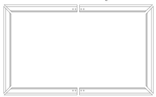
**Step 3.** Both Horizontal Frame parts should each have the *Center Joint (A)* already secured on one side with two *Large Hex Screws (D)*. Insert the *Center Joint (A)* connectors into the other half of the horizontal frame and fasten with two *Large Hex Screws (D)*.
