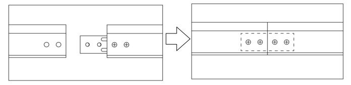
**Step 4.** Insert the *Elbow Joints* (C) to top and bottom sections of the vertical frame. Once inserted, secure the *Elbow Joints* (C) by fastening them with the *Small Hex Screws* (D) and connect the vertical sections to the horizontal frame sections. Make sure all corner frames pieces are flush (no gaps). They should form perfect right angles.
