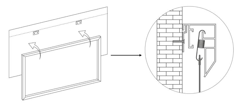
Step 14. Once the top of the frame is secure, slightly push down on the lower portion of the fixed frame into the lower Brackets (F) as shown below. Make sure the frame is secure all around to complete the installation
