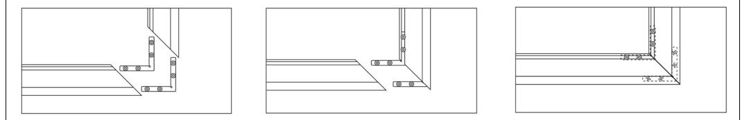
Note: You may have to loosen and adjust the brackets and frame pieces. It will help to leave the screws loose until perfect right angles are formed, then tighten the screws securely.
