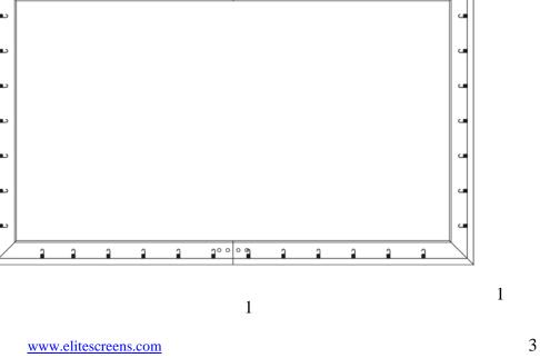
**Step 9.** Two people are suggested for this step. Place the *Center Support Bar (J)* into the top groove on the back of the frame (not the one where the spring inserts) at the approximate center point of the frame. Carefully pull the bottom horizontal frame outward and place the *Center Support Bar (J)* at the approximate center point of the frame. Carefully release the frame once the bar is centered. (See illustrations below for details.)
