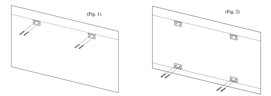
Step 13. Position the fixed frame screen onto the wall Brackets (F) as shown below and push down at the center of the top of the frame to secure.
