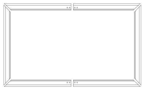
**Step 3.** Both Horizontal Frame parts should each have the *Center Joint* (A) already secured on one side with two *Large Hex Screws* (*D*). Insert the *Center Joint* (A) connectors into the other half of the horizontal frame and fasten with two *Large Hex Screws* (*D*).
