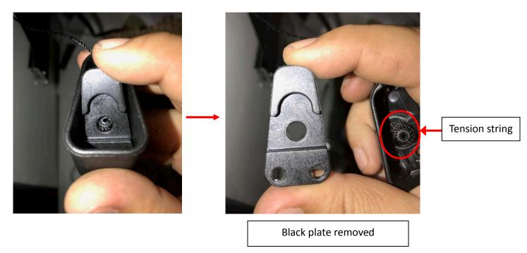
**5.** After unwinding the string, you can pull out the knob. Be aware that the face plate will fall off.
