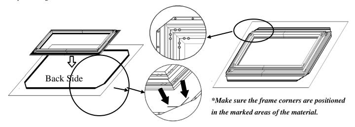
**Step 11:** With one end of the spring and secure inside the groove of the frame, use the *spring hook (d)* to attach the spring to the hole located on the screen material's outer edge in the following order.
