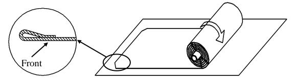
**Step 10:** Carefully and gently place the assembled frame front facing down on top of the screen material. Make sure to not allow the angle edge of the frame to come in direct contact with the screen material to avoid puncturing it.
