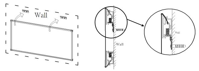
**Step 16:** With the frame slightly tilted outward; connect the bottom brackets onto the bottom groove of the frame. Then secure them by screwing onto the wall
