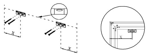
**Step 16**: Position the fixed frame screen onto the top wall brackets as shown below and push down at the center of the top of the frame to secure.
