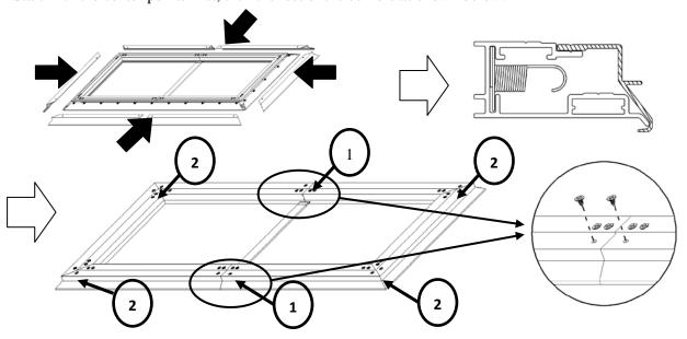
**Step 14**: Install the *angle cover (j)* on each corner of the frame using the M4x7 screws.
