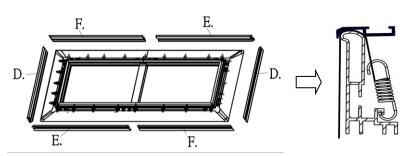
Connect edge trim frames (e/f) together using the M4 center joint (e) and secure with four of the M4x4 screws (m) as show in Step 1. Repeat for other side.
