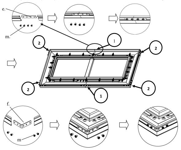
Step 12: Install the *angle cover* (n) on each corner of the frame using the *M4x4 screws* (m).
