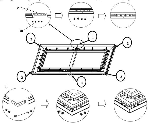
Step 12: Install the *angle cover* (n) on each corner of the frame using the M4x4 screws (m).
