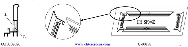
Step 5: Secure the elbow joints by fastening them with M4x7 screws (g), 4 at each corner.
