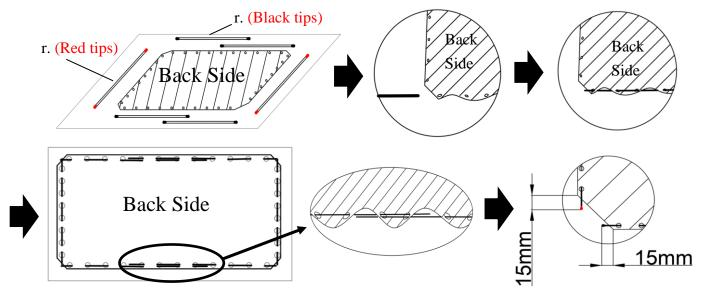
**Step 8:** Carefully and gently place the assembled frame on top of the screen material in the marked areas as shown below. Make sure to not allow the angle edge of the frame to come in direct contact with the screen material to
