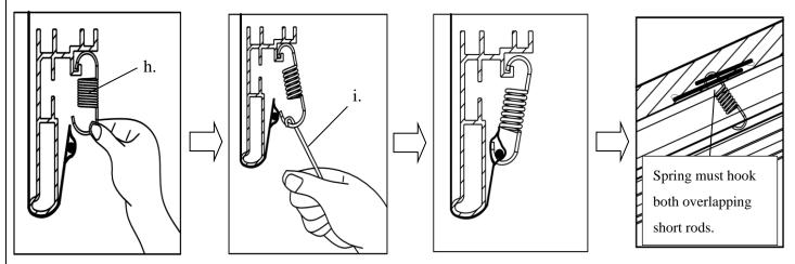
Begin by first attaching the center points on both vertical (left/right) sides, *steps 1-2*. Then the center points on both horizontal (top/bottom) sides, *steps 3-4*. Once all center points have been secured, make sure the screen material is still within the marked areas before proceeding to attach the next springs.
