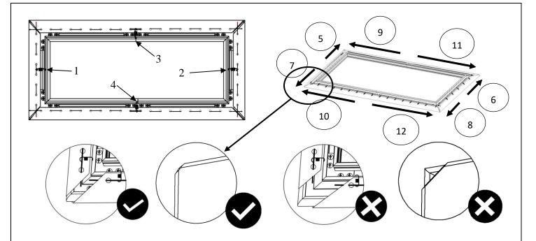
To avoid ripples forming in the material it is imperative that all of the corners are properly wrapped around the edges as illustrated in the check mark diagrams.
