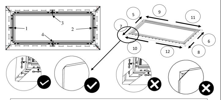
To avoid ripples forming in the material it is imperative that all the corners are properly wrapped around the edges as illustrated in the check mark diagrams.
