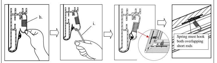
Begin by first attaching the center points on both vertical (left/right) sides, *steps 1-2*. Then the center points on both horizontal (top/bottom) sides, *steps 3-4*. Once all center points have been secured, make sure the screen material is still within the marked areas before proceeding to attach the next springs.
