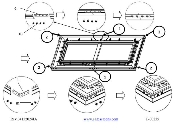
**Step 12**: Install the *angle cover* (*n*) on each corner of the frame using the *M4x4 screws* (*m*). Note: The angle cover screws holes align with the screw holes on the elbow joint.
