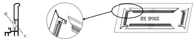
Step 5: Secure the elbow joints by fastening them with M4x7 screws (g), 4 at each corner.
