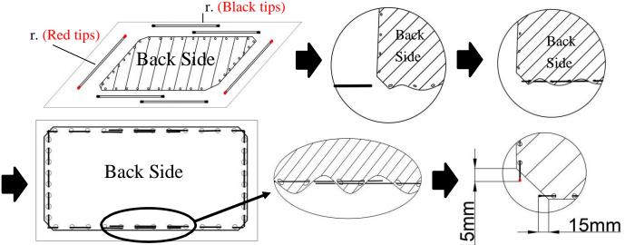
**Step 8:** Carefully and gently place the assembled frame on top of the screen material in the marked areas as shown below. Make sure to not allow the angle edge of the frame to come in direct contact with the screen material to avoid puncturing it.
