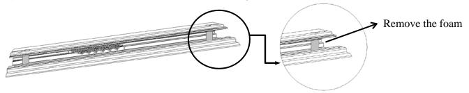
Note: the spring was inserted into the grooves of the frame before shipment already, please make sure to avoid the springs slips out from the grooves, when you remove the foam.
