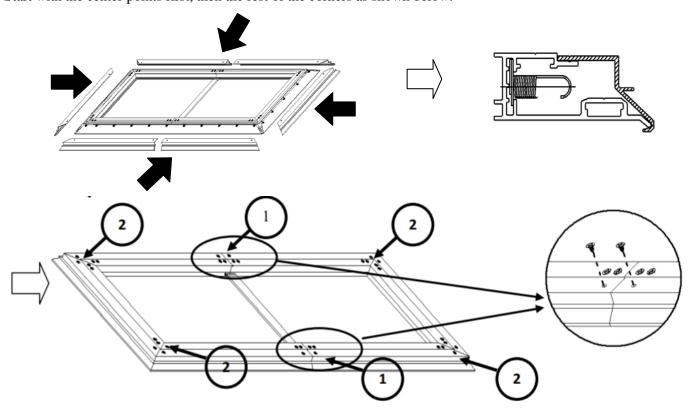
**Step 13**: Install the *angle cover* (j) on each corner of the frame and install the *angle cover clip* (k) to hold down the angle cover.
