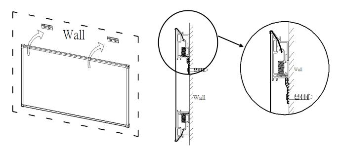
**Step 16:** With the frame slightly tilted outward; connect the bottom brackets onto the bottom groove of the frame. Then secure them by screwing onto the wall.
