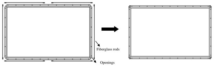
**Step 9:** Carefully and gently place the assembled frame on top of the screen material. Make sure to not allow the angle edge of the frame to come in direct contact with the screen material to avoid puncturing it.
