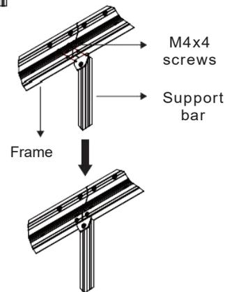
Note: the support bar is mounted in the upper and lower border splicing direction as shown on the right
