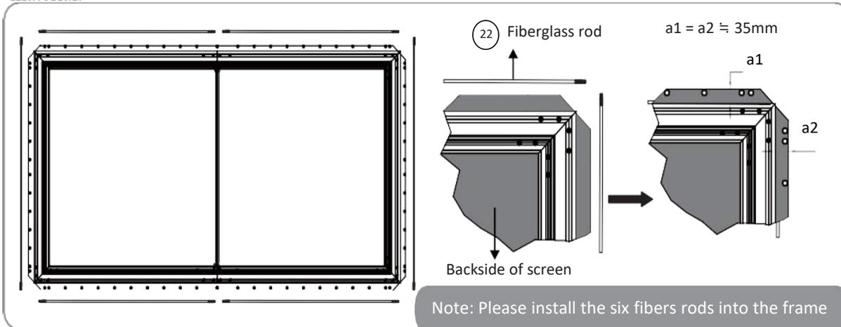
Note: Please install the six fibers rods into the frame
