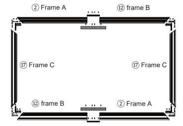
Step 1: Insert the long center joints (a) into each half horizontal frame (A/B) and secure with the screws. These will be the top/bottom frames.
