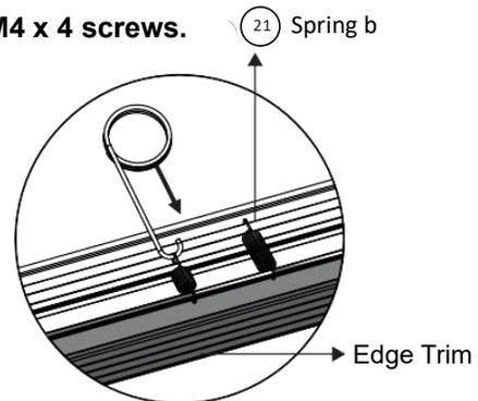
4. Attach a **(21) spring b** on the middle of each edge trim (1-6) to the frame as shown in the illustration.
