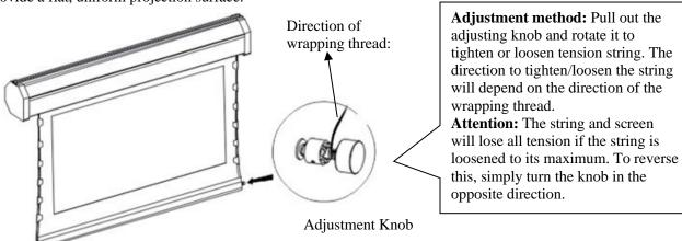
**Attention:** The screen's tension has been preset to achieve its best performance. The adjustments are typically not required. Please contact Elite Screens for assistance to avoid damaging the screen and voiding your warranty.
