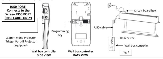
4. Wired 5-12 volt trigger (Fig 3): Requires a 3.5mm to 3.5mm mono cable (not included)
