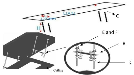
5. Push the screen up into the space. Use the **threaded rods** (C) to attach the screen assembly to the ceiling. The **hexagonal screws** (E) will connect the screen to the rest of the assembly. Once firmly in place; use the **nuts** (F) to ensure a firm connection. Use the **socket wrench** (D) to make sure that the bolts are firmly tightened.
