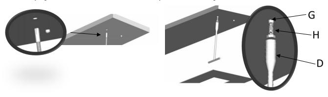
4. Insert the **threaded rods**(C) through the **M8 expanding bolts** and then attach the **M8x40mm hexagonal screws**with the **washer** (E). Last put the **Hanging Bracket** (B) through the threaded rod equal to the height of the screen's housing. Once they are firmly in place (as shown below) make sure that they will hold the weight of the screen.
