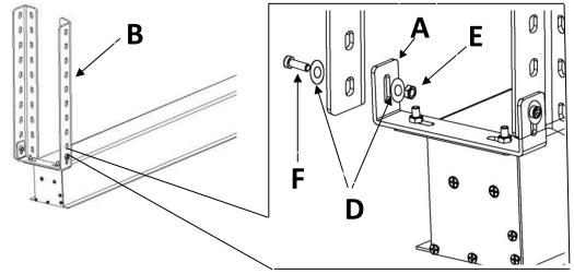
3. Insert the **End Flange piece** (C) on the edge of the housing as shown below to complete the
