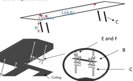
5. Push the screen up into the space. Use the **threaded rods** (C) to attach the screen assembly to the ceiling. The **hexagonal screws** (E) will connect the screen to the rest of the assembly. Once firmly in place; use the **nuts** (F) to ensure a firm connection. Use the **socket wrench** (D) to make sure that the
