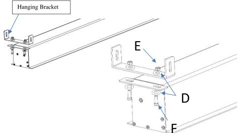
2. Place the **Suspension Bar** (B) over the **Hanging Dracket** (A) and angir with the note as shown below according to the height requirement for your installation area. Secure the **Suspension Bar** (B)
