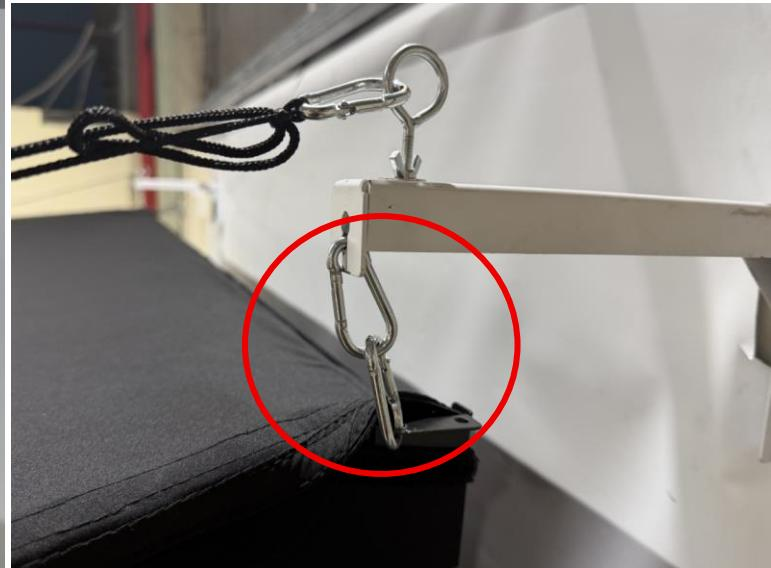
6. Use an M10 wrench (not included) to loosen the upper extend rod of Electric screen (A), turn it out and fix it, and secure the rope to the upper eyebolt of the bracket in a triangular structure.
