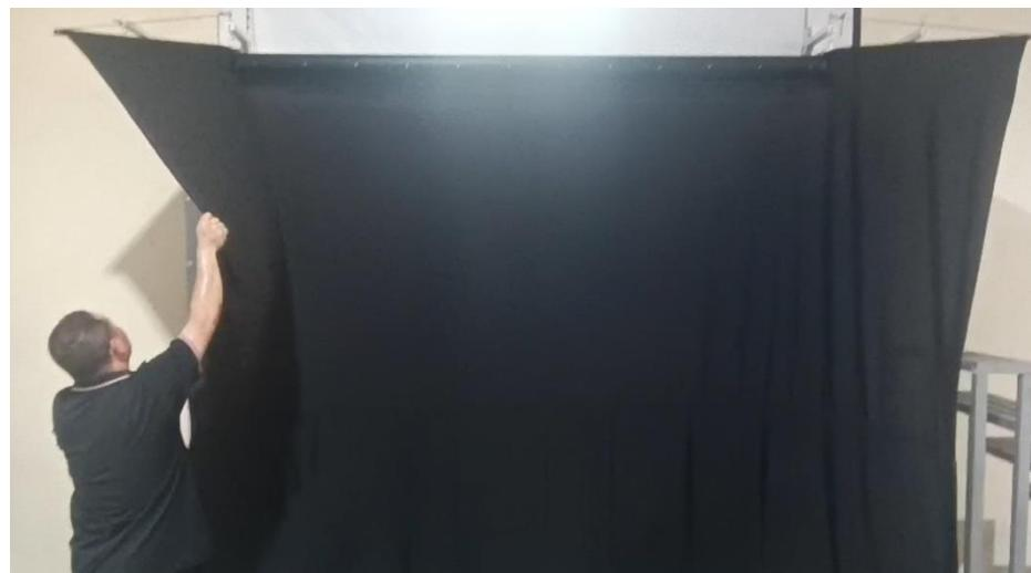
8. Attach Top enclosure cover (C) to the back of Electric screen (A) with Velcro, then pull it flat and attach it to the outer sides of the two upper extended rods.
