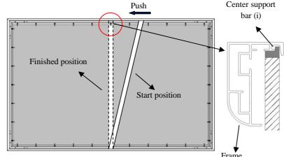
This will provide added stability to your frame and added tension to the material.
