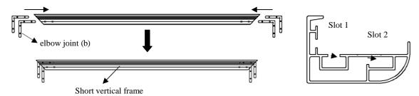
4. Then insert the horizontal long frames into the exposed *elbow joint* (*b*) connectors and fasten them with M5\*6 screws (c).
