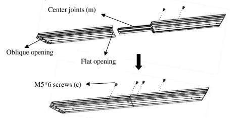
Note: a. Two ½ horizontal long frames should be assembled for a screen.
