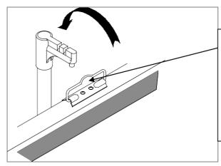
When attaching/detaching the screen to the pull hook, please be sure to raise the screen using the handle indicated here as pulling on other parts of the top support bar may cause damage to the screen. Make sure to firmly hold the handle to avoid the screens from suddenly retracting into the housing.
