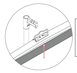
Note: When attaching the screen to the pull hook, you may notice a slight gap between the top bar and screen material. This is completely normal, and it is used to maintain a leveled flat surface when projecting an image.
