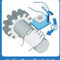
2 Use the pulley to lock the plate
