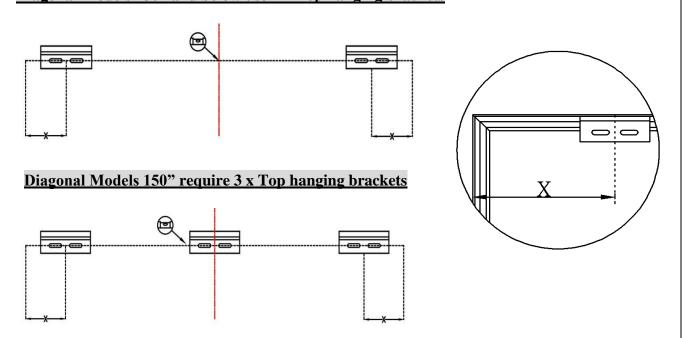
**Step 12:** Position the fixed frame screen onto the top wall brackets as shown below and push down at the center of the top of the frame to secure.
