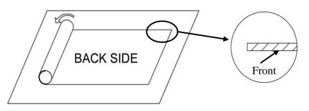
**Step7**: Carefully place the screen on top of the assembled frame as shown below. Make sure that the angular **edges** of the frame are not allowed to come into direct contact with the screen material to avoid puncturing.
