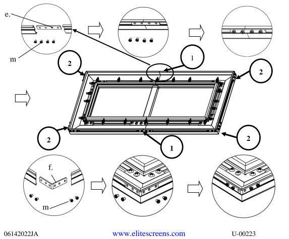
**Step 10**: Install the *angle cover* (*n*) on each corner of the frame using the *M4x4 screws* (*m*). Note: The angle cover screws holes align with the screw holes on the elbow joint.
