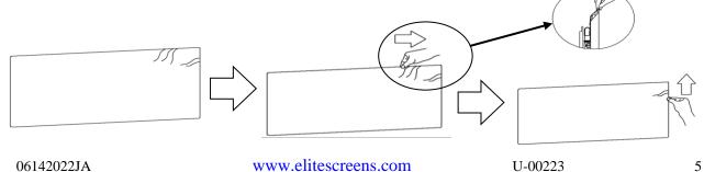
**Incorrect material installation** –The corners of the screen material are not properly wrapped along the edge of the frame leaving the material with unbalanced tension and an uneven finish. To correct, detach springs from material at the corner(s) where material does not lie flat along the edge of the frame, reposition the material so that it lies flat and wraps along the edge of the frame, and reattach springs to the material.
