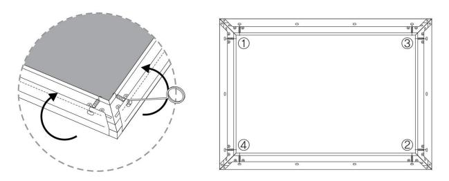
Step 7. Once the material is completely attached, place the black *rubber end caps* (J) at each of the *tension rod* (H) ends.
