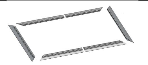
**Step 3.** Insert the *Center Joint (A)* connectors into one-half of the horizontal frame and secure with 4 (*M5x10mm*) screws. Once secure, connect the other half of the horizontal frame and fasten with 4 more screws.
