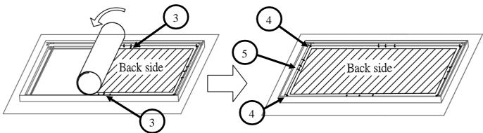
**Step 9.** Attach the vertical portions of the material, begin in the center, and move towards the corners (6). Lastly, connect the horizontal sections of the material by connecting the center of the material and make your way towards the corners (7).
