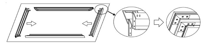
**Step 7.** Secure the elbow joints by fastening them with 4 M4x6 screws (4 at each corner). Do no tighten completely until all frame pieces are assembled correctly.
