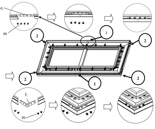
**Step 10**: Install the *angle cover* (n) on each corner of the frame using the *M4x4 screws* (m).
