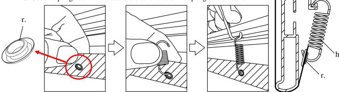
Begin by first attaching the center points on both vertical (left/right) sides, *steps 1-2*. Then the center points on both horizontal (top/bottom) sides, *steps 3-4*. Once all center points have been secured, make sure the screen material is still within the marked areas before proceeding to attach the next springs. Continue attaching the rest of the springs to the material in the following order in *steps 5-12*.
