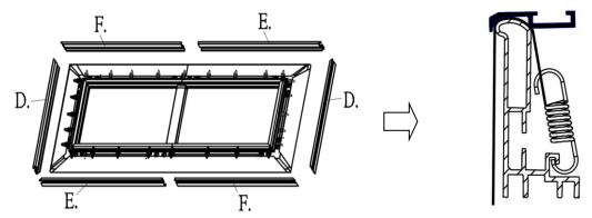
Connect edge trim frames (e/f) together using the M4 center joint (e) and secure with four of the M4x4 screws (m) as show in Step 1. Repeat for other side.
