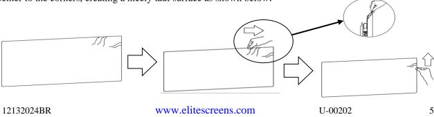
**Incorrect material installation** –The corners of the screen material are not properly wrapped along the edge of the frame leaving the material with unbalanced tension and an uneven finish. To correct, detach springs from material at the corner(s) where material does not lie flat along the edge of the frame, reposition the material so that it lies flat and wraps along the edge of the frame, and reattach springs to the material.
