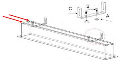
2. Place the Suspension Bar (D) on the Hanging Bracket (C) and align with the hole as shown below. Secure the Suspension Bar (D) with the Hex Screw (B), Washer (E) and the Hex Nut (F). Install the Suspension Bars (D) to your ceiling according to their distance.
