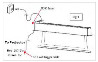
6. <u>Wireless 5-12 volt trigger</u> (Item F, Fig 5): The RF remote control serves as a dual purpose, independently as a handheld remote control, or in conjunction with the Wireless 5-12 volt trigger cable. The radio frequency technology can be programmed to send a wireless signal to synchronize its drop/rise with the projector's power cycle.
