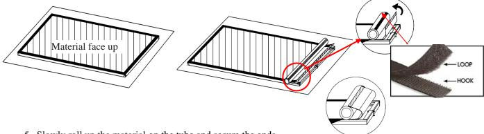
5. Slowly roll up the material on the tube and secure the ends.
