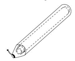
7. Once the material has been completely rolled, insert the rolled material with the outer tube lying horizontally. DO NOT force it in as that will crush the ends and damage the material.
