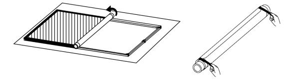
6. Then insert the material rolled on the tube into the bag.
