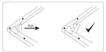
10. Press the locking buttons, near the folding joints, and slowly gather the sides of the folding frame.
