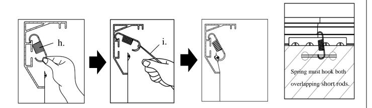
First connect on four corners, steps 1-4. make sure all four corners are fixed before proceeding with next spring.
