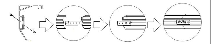
**Step 4:** Connect the *elbow joints* (*c/d*) to the top and bottom sections of the vertical frame. Once inserted, connect the vertical sections to the horizontal frame sections. Make sure all holes are in alignment and the frame pieces are flush (no gaps). They should form perfect right angles.
