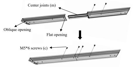
Note: a. Two ½ horizontal long frames should be assembled for a screen.
