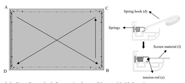
Next, attach the Center Support bar before securing the rest of the material with the springs.
