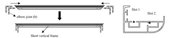
4. Then insert the horizontal long frames into the exposed *elbow joint* (b) connectors and fasten them with M5\*6 screws (c).
