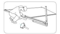
5. Next, screw the *eyebolts* (*F*) into the openings located at the top of the frame (Fig.11).
