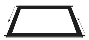
10. Tie 4 pieces of *rope* (2 on the left and 2 on the right) to the *eyebolts* (*F*) that are located at the top of the frame. Next, lift the screen up while simultaneously opening the frame legs. Two people are needed for this step. Fig.17-18
