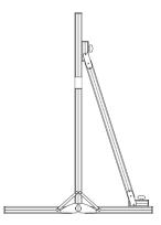
12. To secure the frame, place a *stake* (*I*) into each hole located on the frame footing, and hammer it into the ground. Finally, tie the 4 *ropes* (*G*) to the stakes to prevent the screen from tilting or falling over. As shown in fig.19.
