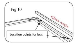
3. Once you have aligned the leg's holes with the frame's holes, secure with the knob screws.
