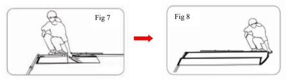
2.Once the screen material is fully extended, secure the material by snapping the buttons onto the frame studs. Fasten the buttons in the following order as shown on **Fig. 9**.
