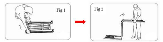
Next, unfold the frame until the latch on the hinge "clicks" into place. Repeat the procedure for the shorter sections, as shown below.
