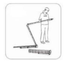
2. Lay the frame on its backside on clean surface, then lay the legs over on the frame in the position desired.
