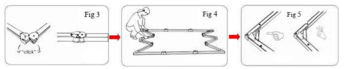
Note: When unfolding the frame and legs, be sure the latches on the hinges "click" into place. Please also make sure all 4 corners of the frame are at a 90° angle and the hinged support bar is straight and not bent.
