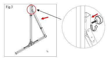
4. Lastly, make sure your screen is secure and stable. Make any adjustments if needed. The installation is now complete. *Note: Refer to Yard Master 2 User Guide for additional steps on securing your screen.*
