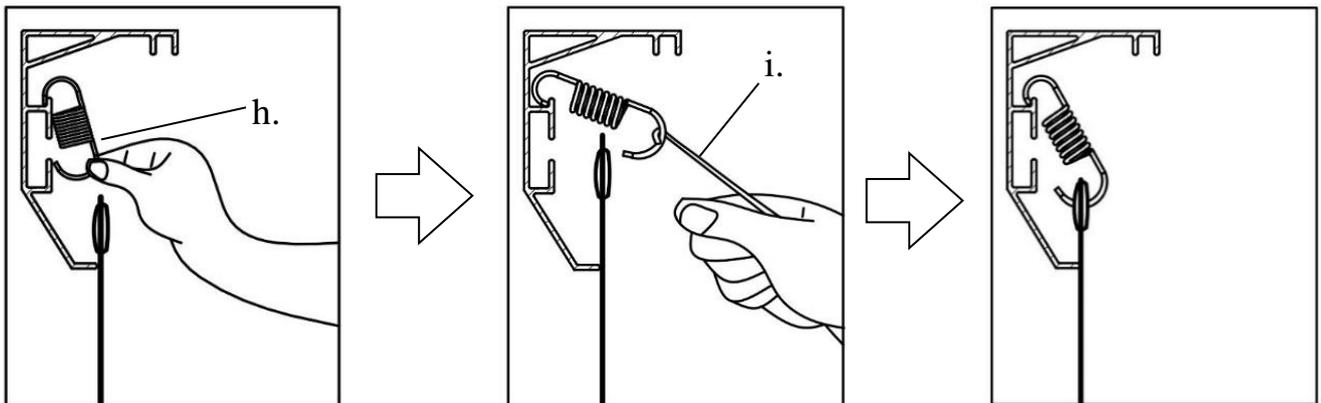
First connect on four corners, steps 1-4. make sure all four corners are fixed before proceeding with next spring.
