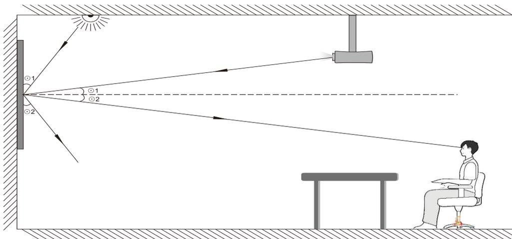
**Projector Tabletop:** Make sure the projector (*light in*) is angled ( $\Theta 1$ ) to reflect ( $\Theta 2$ ) at the mirror-opposite angle (*light out*) to align with the viewer's eye level.
