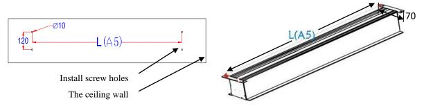
3. The **M8expanding bolts** (G) mount into thick wood beams, stone or concrete and will support the screen. Use the **Socket wrench** (D) to attach the **M8x40mm hexagonal screws**. The expanding bolts should be firmly tightened and tested to make sure that they will hold the weight of the screen.
