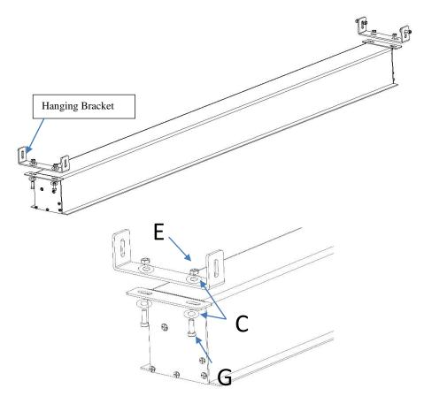
Place the Suspension Bar (B) over the Hanging Bracket (A) and align with the hole as shown below according to the height requirement for your installation area. Secure the Suspension Bar (B) with the M6x20mmScrew (B), M6x13mmx2mmWasher (E) and the M6 Nut (F). Repeat the process for the other side.
