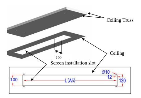
2. Drill 4 holes in the ceiling that correspond with the attachments on the various casing sizes. The width should be 120mm. The length of (A5) in the diagram below depicts the distance between the holes located on each ear end of the screen's case.
