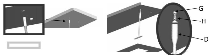
4. Insert the **threaded rods**(C) through the **M8 expanding bolts** and then attach the **M8x40mm hexagonal screws**with the **washer** (E). Last put the **Hanging Bracket** (B) through the threaded rod equal to the height of the screen's housing. Once they are firmly in place (as shown below) make sure that they will hold the weight of the screen.
