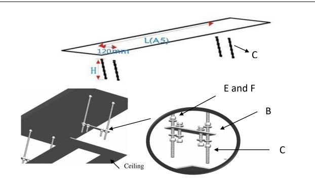
5. Push the screen up into the space. Use the **threaded rods** (C) to attach the screen assembly to the ceiling. The **hexagonal screws** (E) will connect the screen to the rest of the assembly.Once firmly in place; use the **nuts** (F) to ensure a firm connection. Use the**socket wrench** (D) to make sure that the bolts are firmly tightened.
