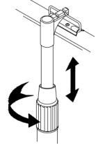
2. Lift the support handle up and out of the "notches" and guide the material back down into the casing. Release the handle when the screen material has fully retracted.
