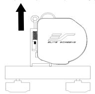
Lift screen assembly up and away from the base foot
