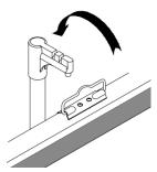
4. Twist the locking ring counter-clockwise to loosen the telescoping function of the upright support and raise the screen to its desired level.
