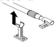
2. Insert the upright support into the socket on the center base foot.
