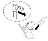
3. Hang the suspension handle of the screen from either of the notches of the upright support.
