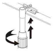
5. Rotate the locking ring clockwise to lock the upright support at its desired height setting.
