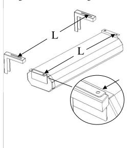
2. Measure and mark the height required for your installation. Next, drill three holes vertically 37mm apart for the 6 inch wall brackets (E). Then, drill another hole according to the measurement distance obtained from Step 1. Finally, drill the remaining two holes for the wall bracket.
