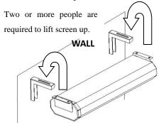
5. Align the screw holes from the screen's end flanges to the wall brackets top opening.
