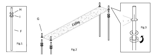
5. Lastly, align the end flange holes to the threaded support rods and fasten them with the nuts and washers as show below.
