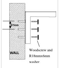
4. After securing the 6 inch wall brackets (E)to the wall, bring the screen over the top of the brackets.
