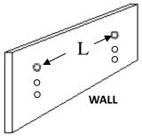
3. Insert the *hollow wall*Anchors (A) into the drilled holes. Align the 6 inch wall brackets (E) to the drilled holes and secure with the screws (B).
