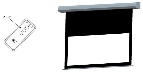
Press the **16:9** button on the RF remote, this will retract the 2.35:1 screen into the housing. When the 2.35:1 screen has stopped, the 16:9 screen commences its deployment.
