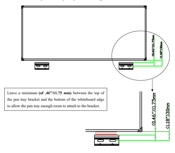
**Step 5:** Attach the pen tray on the tray hanging bracket as shown in the steps below.
