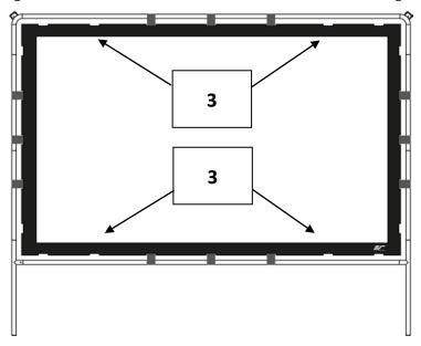
3. Leaving the corner sections for last, attach the remainder of the top and bottom material with the *velcro bands*, using one person on each side to maintain even tensioning and a centered screen.
