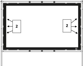
2. Next, with one person at each side, attach the left and right sides of the material with the *velcro bands*, starting with the 3 middle sections.
