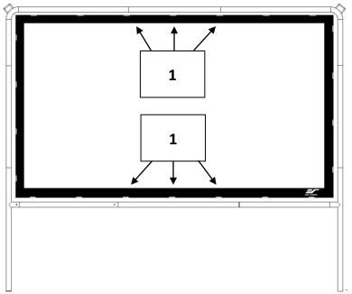
1. With one person at the top of the frame and the other at the bottom, begin by attaching the material with the *velcro bands*, starting at the 3 middle sections keeping the material centered and evenly tensioned.
