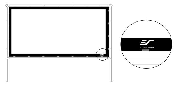
5. Attach the screen material by the exposed areas of the vertical and horizontal support rods onto the metal frame wrapping the velcro bands around the rod and frame. **Two people are recommended for the following steps.**
